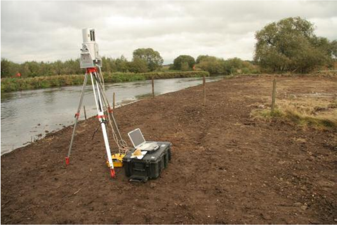
Day 22. Laser Scanner for baseline geomorphological assessment conducted by JBA Consulting and the University of Salford.
