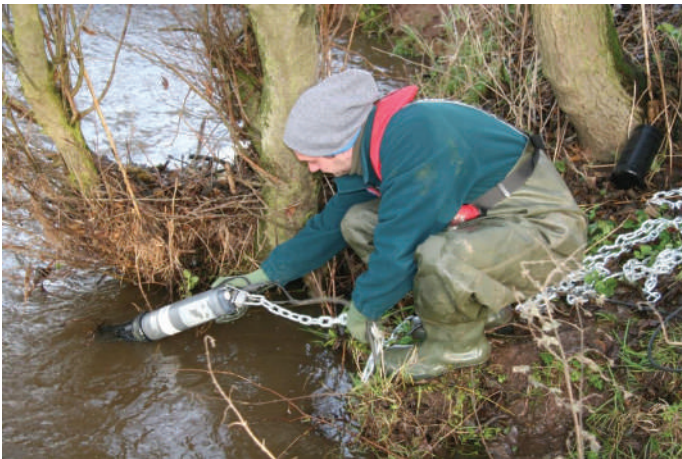
A Sonde (remote water quality recording unit) being positioned by EA staff on the upper Gayton Brook.
