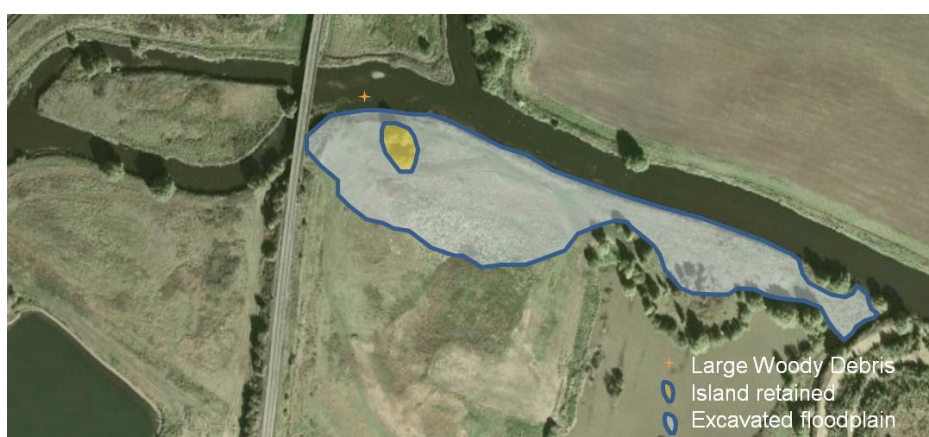
Figure 1 Location of floodplain excavation works on the River Trent at Croxall Lakes.
